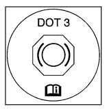
Your brake master cylinder reservoir is filled with DOT-3 brake fluid. See Engine Compartment Overview on page 308 for the location of the reservoir.
